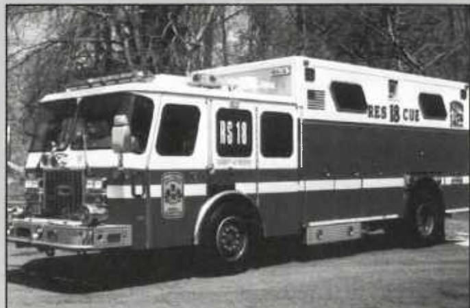
In 1984 and 1986, Fairfax County purchased squads built on Ford C chassis. The 1984 truck was sent back to Emergency One in 1995 and received a brand new Emergency One Protector cab and was placed in service as Rescue Squad 18. The 1986 squad had a similar conversion and is in service at Station 26. (Mike Sanders photo).
