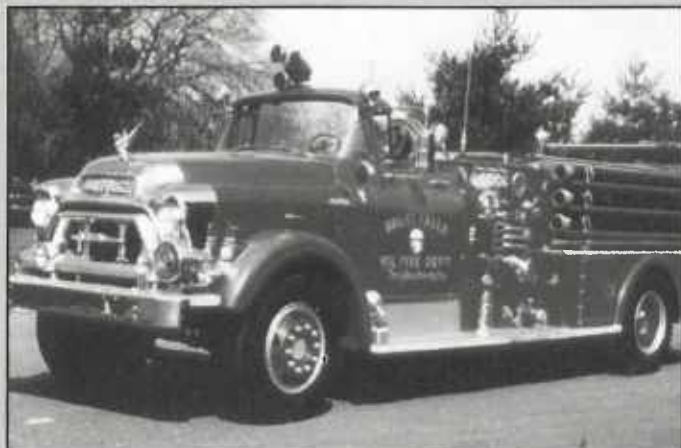
Great Falls Company 12 ran this nice 1955 open cab GMC/American pumper, complete with plenty of front end chrome, a roto ray warning light above the cab, and a 750 gpm pump. (Mike Sanders photo).
