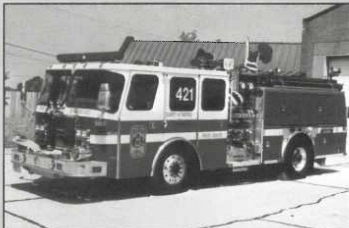
Engine 421 is a representation of the current type of county purchased engines. This 1998 Emergency One Cyclone model as a 1250 gpm pump and carries 750 gallons of water. (Mike Sanders photo).
