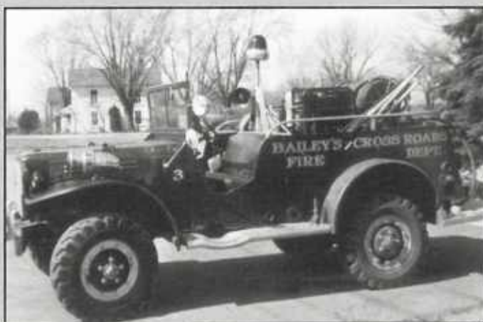
Bailey's Cross Roads purchased an old army weapons carrier and transformed it into a field brush truck. This truck was a 1945 Dodge. (Pete West photo).
