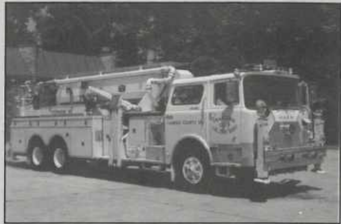
Franconia's 1973 Mack CF 75' aerialscope was one of the first Mack tandem rear axle aerialscope produced. The addition of a 150 gallon water tank created the need for tandem rear axles. (Mike Sanders photo).
