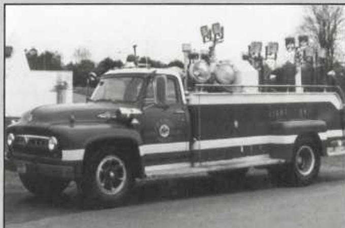
This 1953 Ford light unit was once Penn Daw's pumper that had a 750 gpm pump and a 500 gallon water tank. A 1956 Ford once belonging to Vienna had a similar conversion to a light unit. Shown above is Light Unit 9. (Mike Sanders photo).
